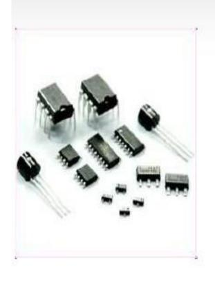
When the input and output relationship of a circuit is linear, *linear ICs* are used. Input and output can take place on a continuous range of values.
