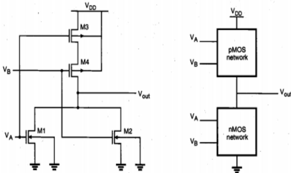
Fig. (Two-Input NOR) Gate.
