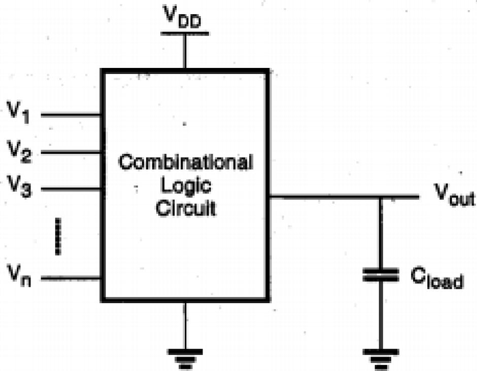
Fig. Generic combinational logic circuit (gate).
