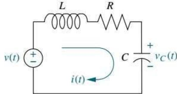
Summing the voltages around the loop, assuming zero initial conditions, yields the integro-differential equation for this network as
