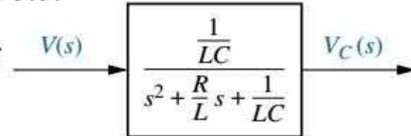
$$LC \frac{d^2v_C(t)}{dt^2} + RC \frac{dv_C(t)}{dt} + v_C(t) = v(t) \Rightarrow (LCs^2 + RCs + 1)V_C(s) = V(s)$$
