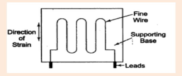
A tensile stress tends to elongate on the wire and thereby increase its length and decrease its cross-sectional area. The combined effect is increase in resistance.
