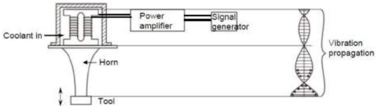
Working of horn as mechanical amplifier of amplitude of vibration
