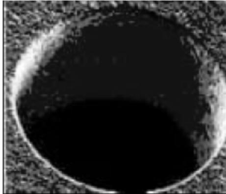
Figure 2: A non-round hole made by USM
