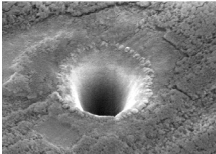
Figure 18: SEM micrograph hole drilled in 250 micro meter thick Silicon Nitride with 3<sup>rd</sup> harmonic Nd: YAG laser
