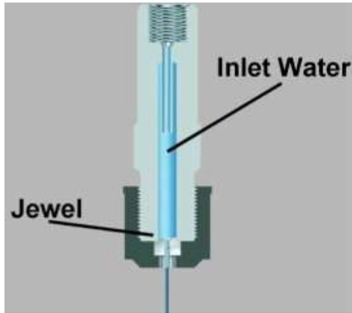
Figure 3: Water jet cutting
