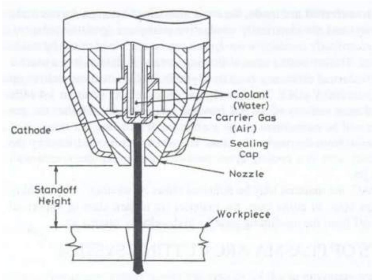
**Fig. 9.2** Details of air plasma torch construction [*Benedict, 1987*;
