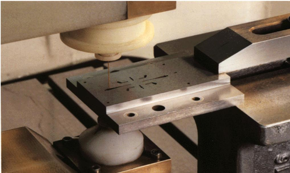
Figure 15: Wire erosion of an extrusion die
