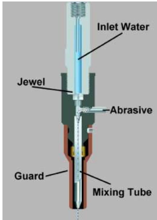
Figure 4: Abrasive water jet machining
