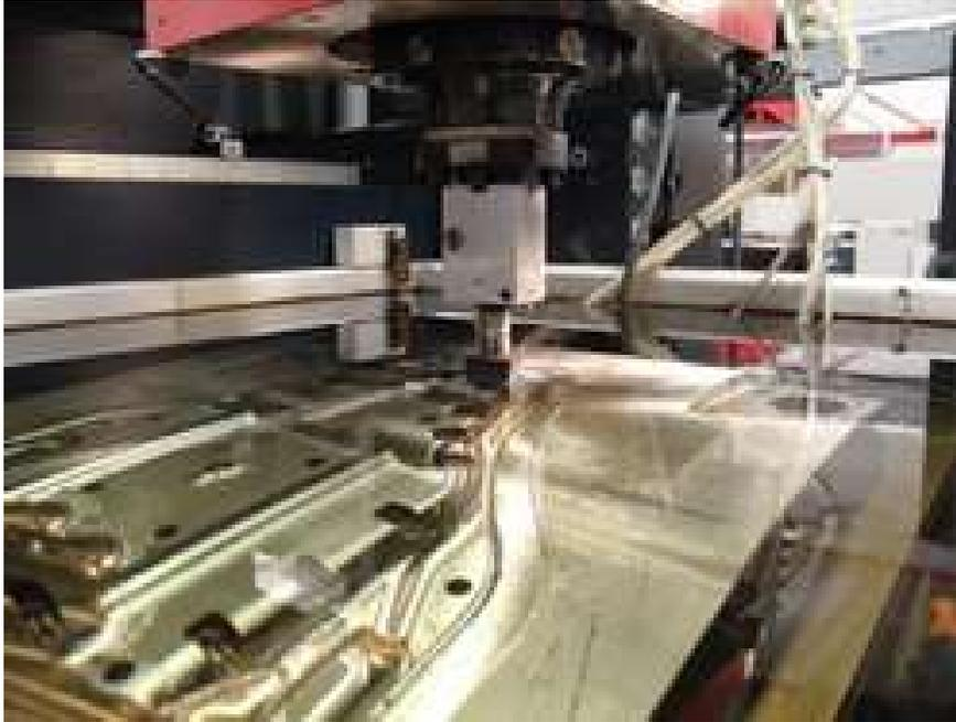
Figure 12: Electrical discharge machine
