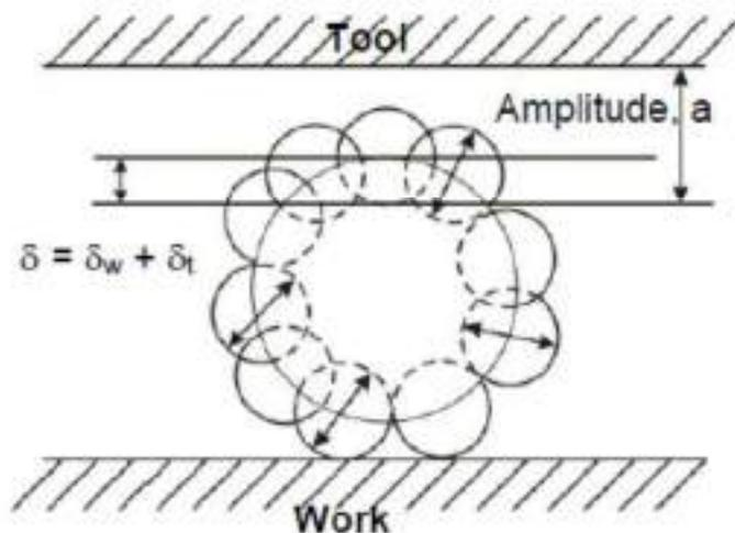
Interaction between grit and workpiece and tool to depict the workpiece and tool deformations
