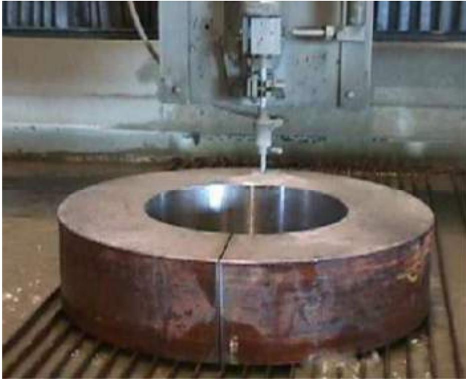
Figure 5: Abrasive water jet cutting
