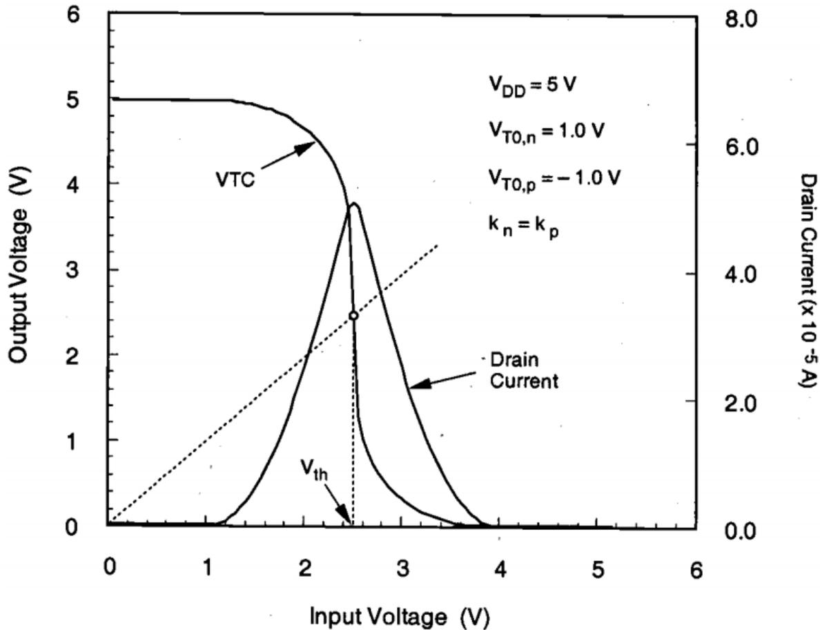
**Fig.** Typical VTC and the power supply current of a CMOS inverter circuit.
