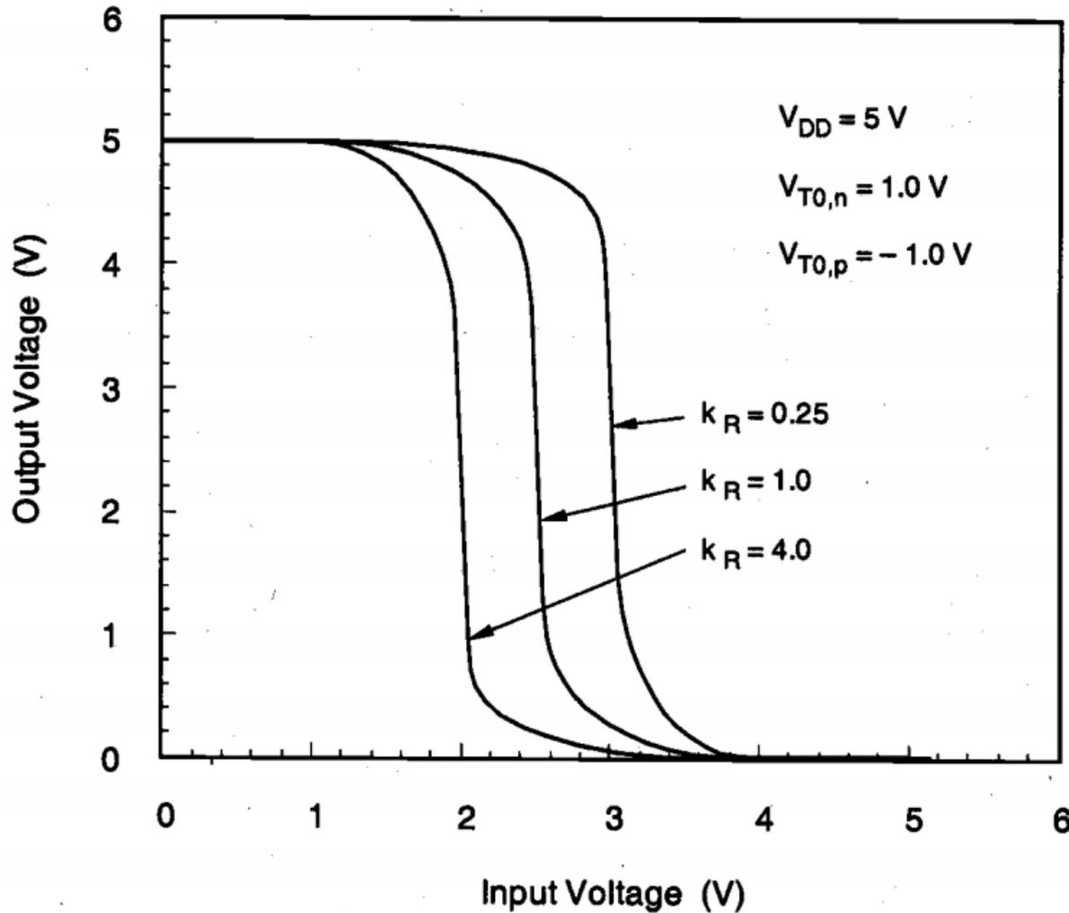
**Fig.** Voltage transfer characteristics of three CMOS inverters, with different NMOS-to-PMOS ratios.
