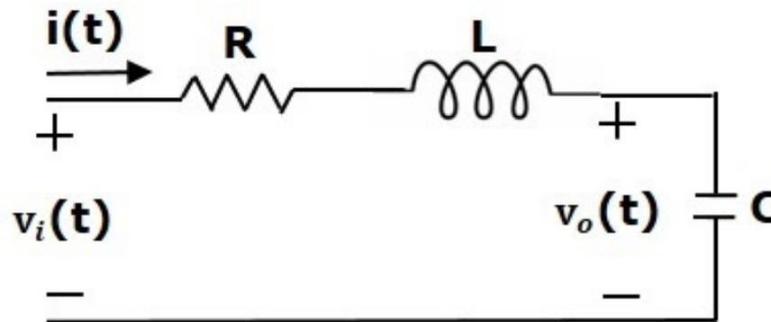
There are two storage elements (inductor and capacitor) in this circuit. So, the number of the state variables is equal to two and these state variables are the current flowing through the inductor,  $i(t)$  and the voltage across capacitor,  $v_c(t)$  .
