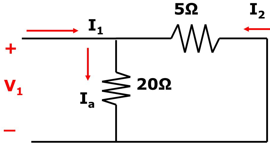
$$V_1 = 20I_a \dots\dots(1)$$
