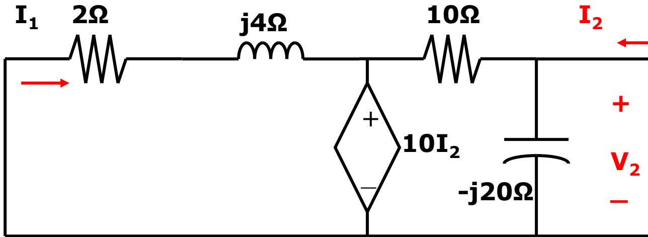
$$I_1 = \frac{-10I_2}{2 + j4} \dots\dots(1)$$
