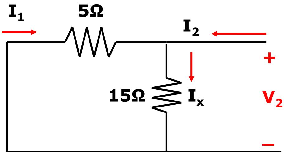
$$V_2 = 15I_x \dots\dots(3)$$
