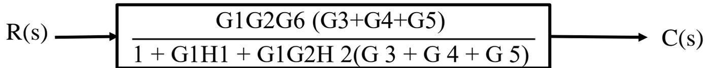
$$\frac{C(s)}{R(s)} = \frac{G1G2G6 (G3+G4+G5)}{1 + G1H1 + G1G2H2(G3 + G4 + G5)}$$
