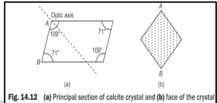
Fig. 14.12 (a) Principal section of calcite crystal and (b) face of the crystal
