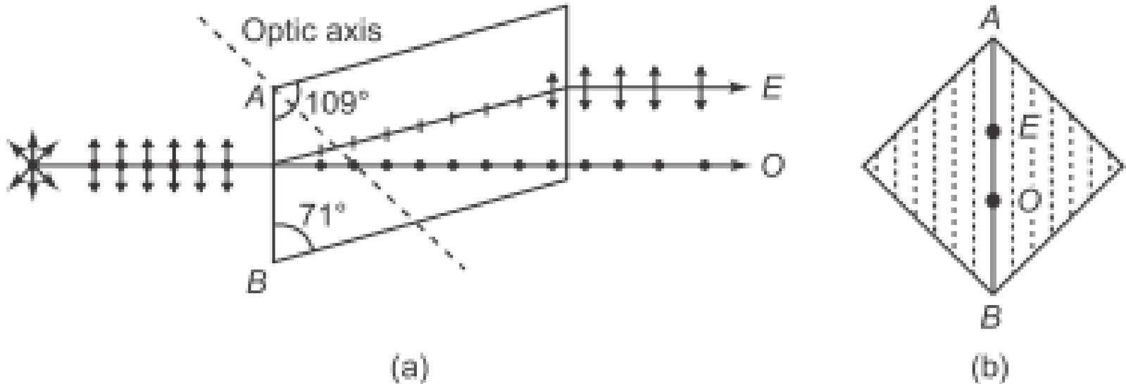
**Fig. 14.13** (a) Double refraction of unpolarised light and (b) dots showing the images corresponding to E-and O-rays
