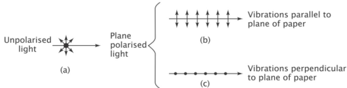
**Fig. 14.5** (a) Unpolarised light and (b, c) linearly polarised light
