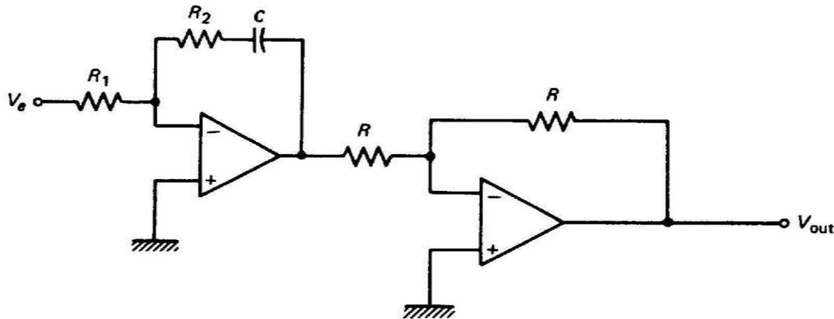
$$V_{out} = \left(\frac{R_2}{R_1}\right)V_e + \left(\frac{R_2}{R_1}\right)\frac{1}{R_2 C} \int_0^t V_e dt + V_{out}(0)$$
