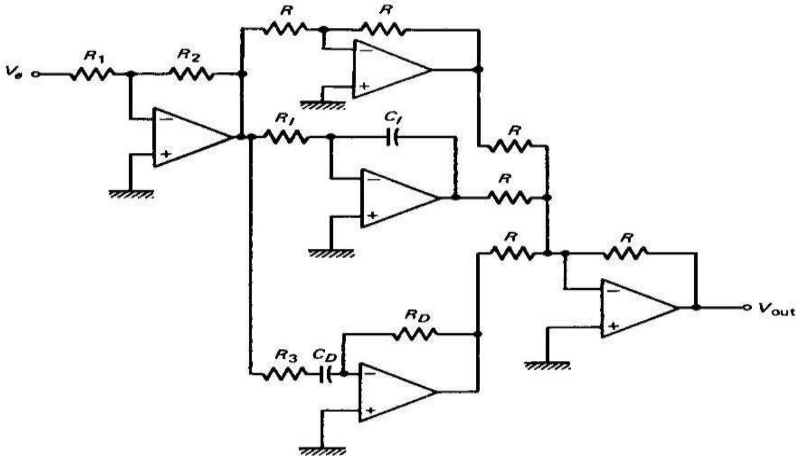
$$-V_{out} = \left(\frac{R_2}{R_1}\right)V_e + \left(\frac{R_2}{R_1}\right)\frac{1}{R_I C_I} \int V_e dt + \left(\frac{R_2}{R_1}\right)R_D C_D \frac{dV_e}{dt} + V_{out}(0)$$
