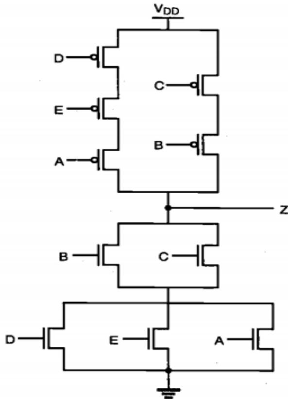
$$\begin{aligned} \left(\frac{W}{L}\right)_{n,eq} &= \frac{1}{\frac{1}{\left(\frac{W}{L}\right)_D + \left(\frac{W}{L}\right)_E + \left(\frac{W}{L}\right)_A} + \frac{1}{\left(\frac{W}{L}\right)_B + \left(\frac{W}{L}\right)_C}} \\ &= \frac{1}{\frac{1}{30} + \frac{1}{20}} = 12 \end{aligned}$$
