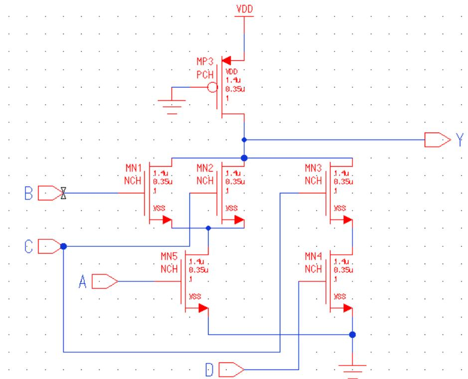
Fig. using Pseudo NMOS logic
