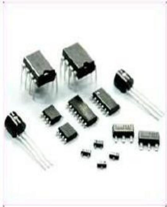
When the input and output relationship of a circuit is linear, *linear ICs* are used. Input and output can take place on a continuous range of values.
