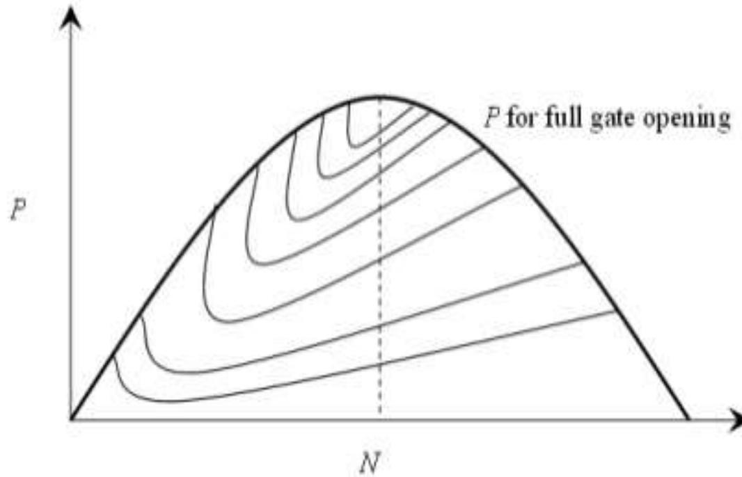
Constant Efficiency curves for Reaction turbine
