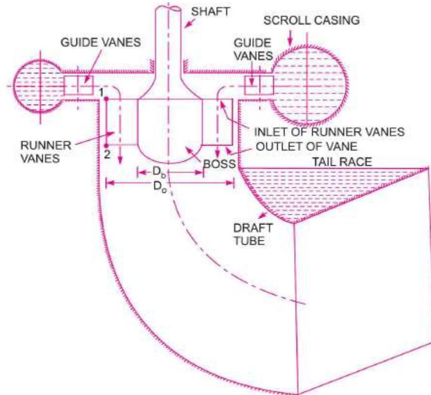
Fig. Main components of Kaplan turbine.
