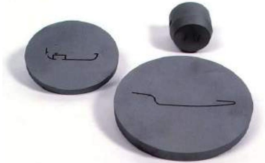
Figure 16: Sparked eroded extrusion dies
