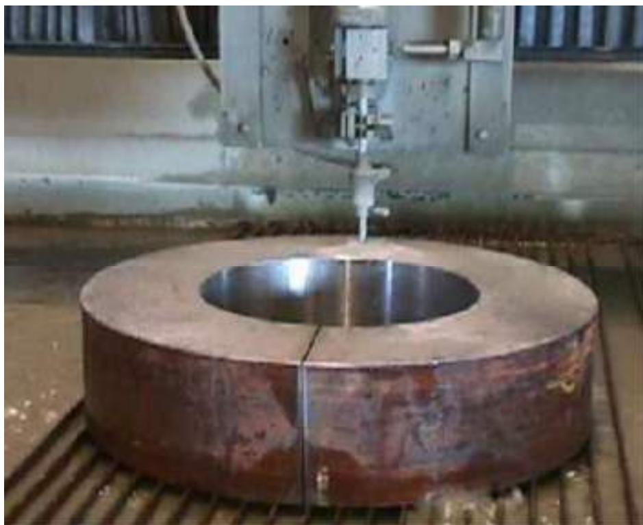
Figure 5: Abrasive water jet cutting
