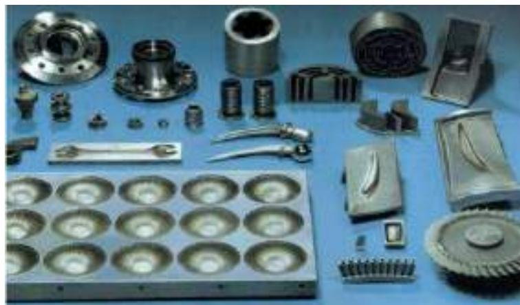
Figure 9: Parts made by ECM
