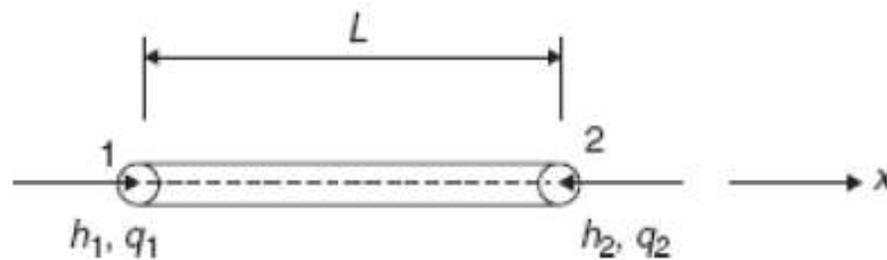
Figure- 1-D Fluid flow element
