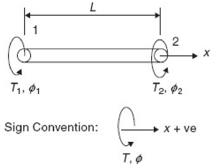
Fig. 1-D Torsion element
