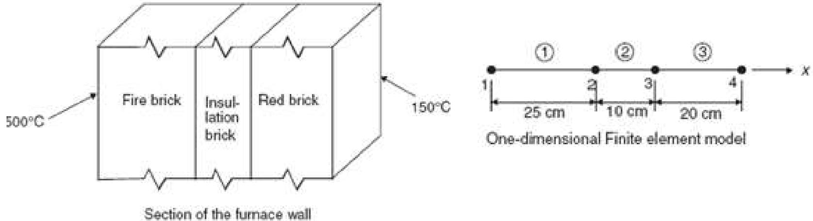
Figure 1 Cross section of furnace wall and its finite element model
