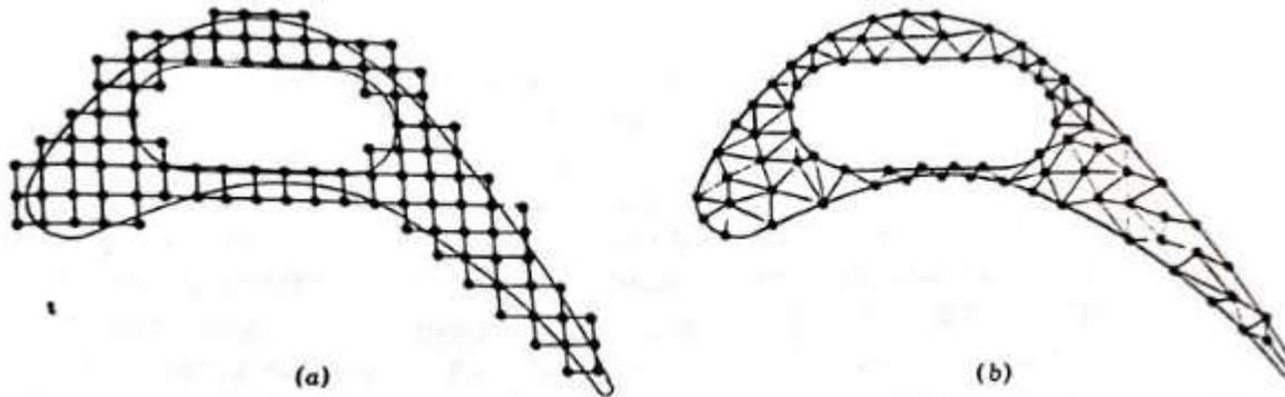
Fig. FEM and FDM discretization of turbine blade profile (a) typical FEM discretization (b) typical FDM discretization
