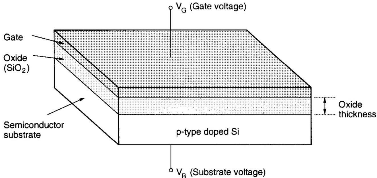
**Figure 3.1** Two-terminal MOS structure.
