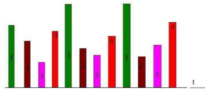
Fig: 2.23 Multiplexing of FOUR signals.
