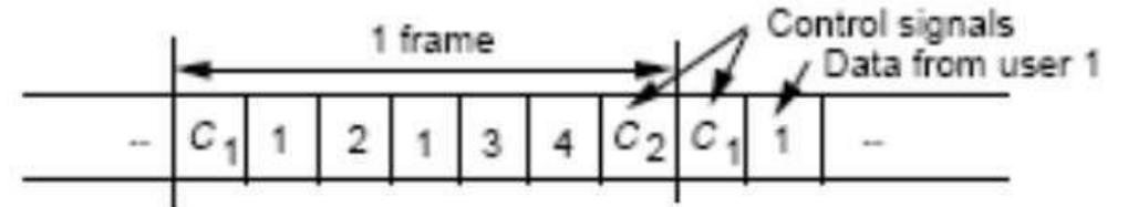
A Typical Framing Structure for TDM
