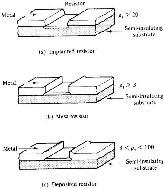
**Figure 12-4-1** Configurations of planar resistors.
