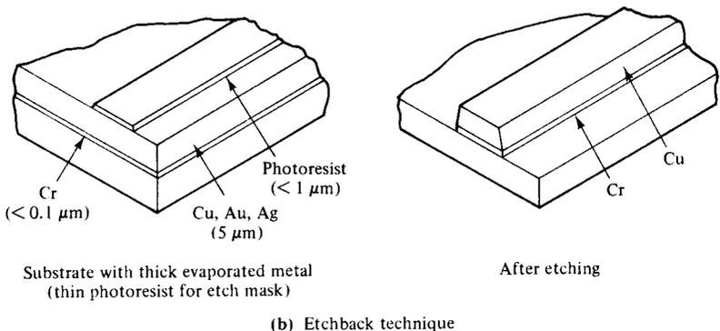
**Figure 12-5-1** Fabrication of hybrid ICs. (After M. Kumar and I. J. Bahl [13]; reprinted by permission of John Wiley & Sons.)
