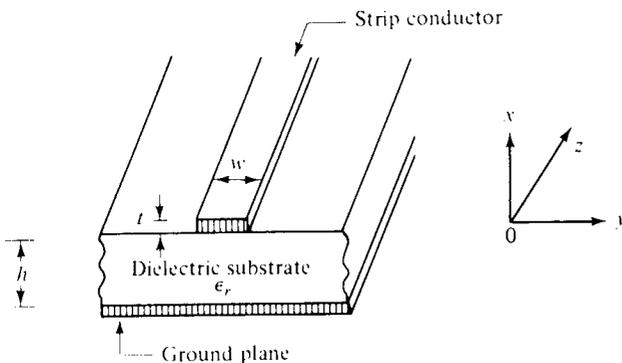
**Figure 11-1-4** Schematic diagram of a microstrip line.
