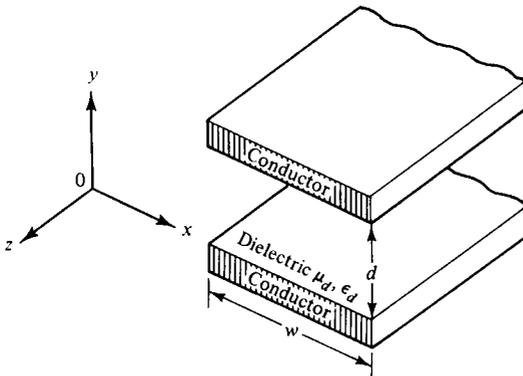
**Figure 11-2-1** Schematic diagram of a parallel strip line.
