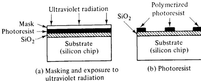
**Figure 12-2-1** Photoetching process.
