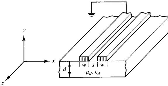
**Figure 11-3-1** Schematic diagram of a coplanar strip line.
