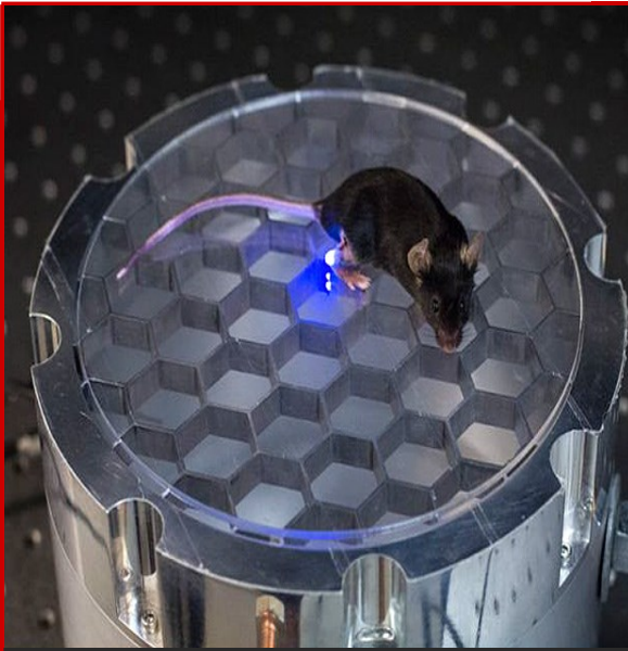
Mouse's body transmitting energy to an implantable device that delivers light to stimulate leg nerves in an optogenetics project.
