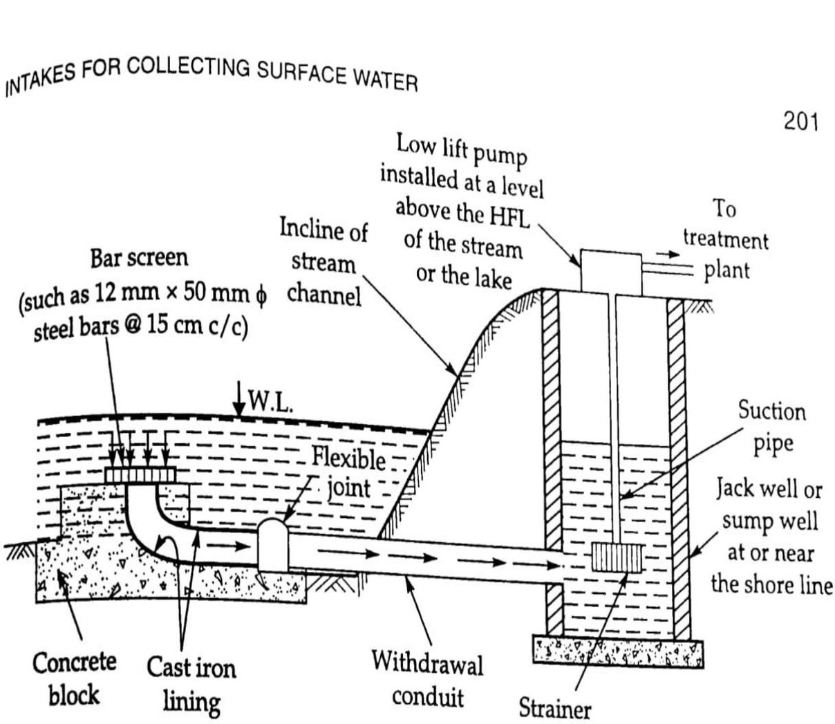
Fig. 5.1. Simple concrete block—submerged intake.
