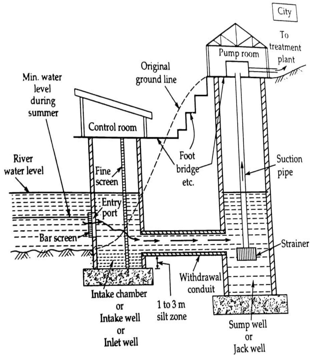
Fig. Section of a typical twin well type of a river intake
