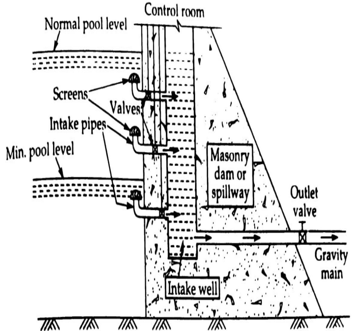
Fig. intake well or valve tower for concrete gravity or masonry dams
