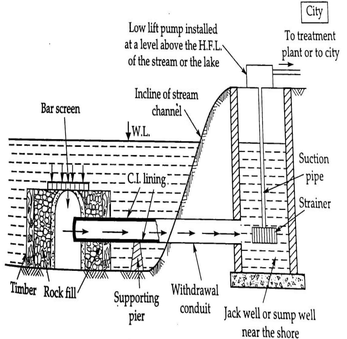
Fig. 5.2. Rock filled timber crib—submerged intake.
