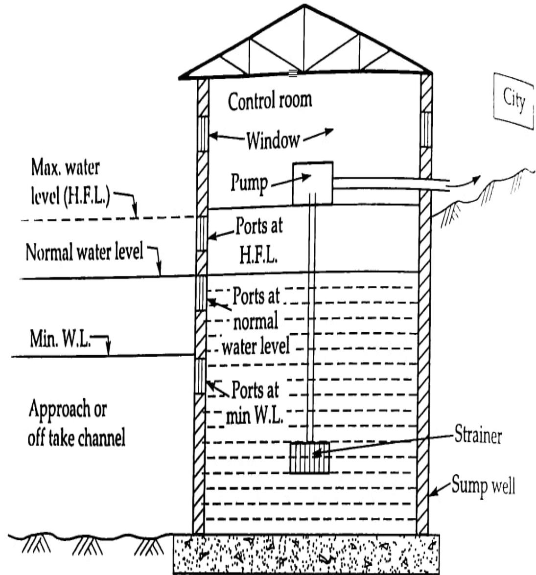
Fig. Single well type of a river intake structure
