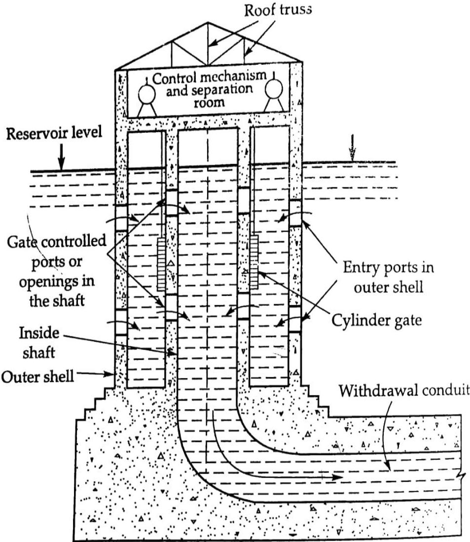
Fig. 5.3. Wet intake tower standing in the river or reservoir.
