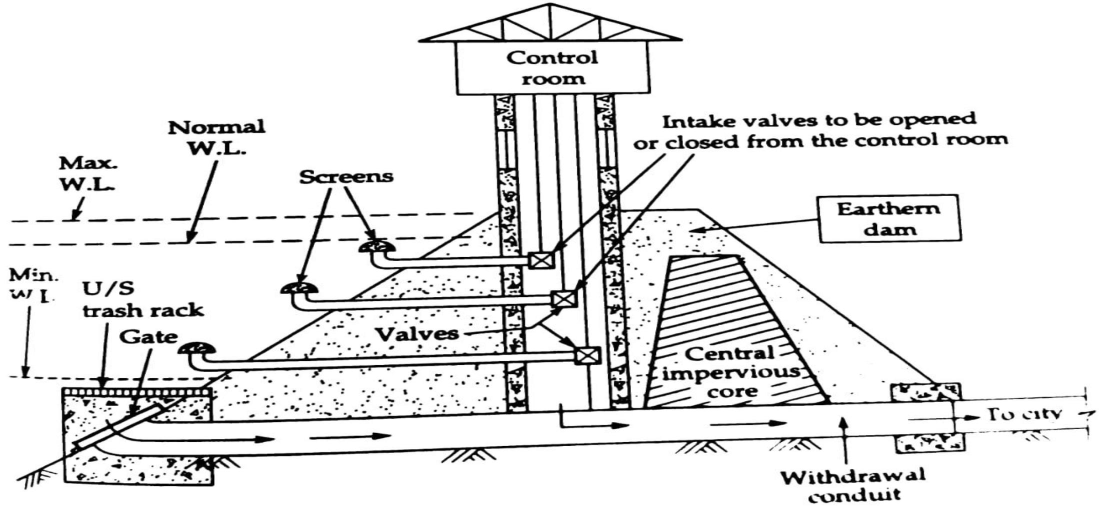
Fig. Valve Tower situated within an earthen dam
