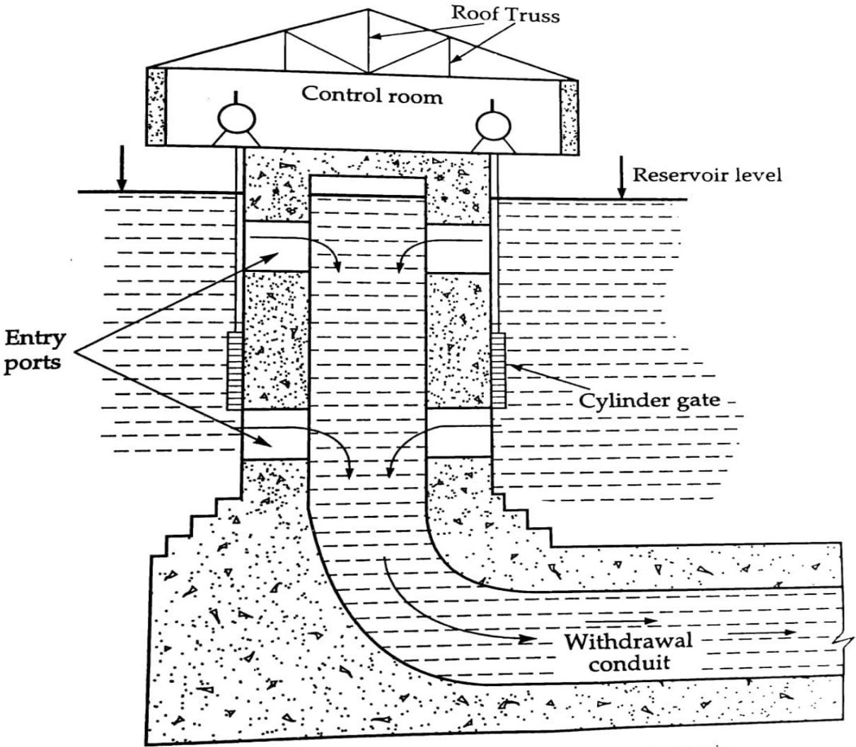
Fig. 5.4. Dry intake tower standing in the river or reservoir.
