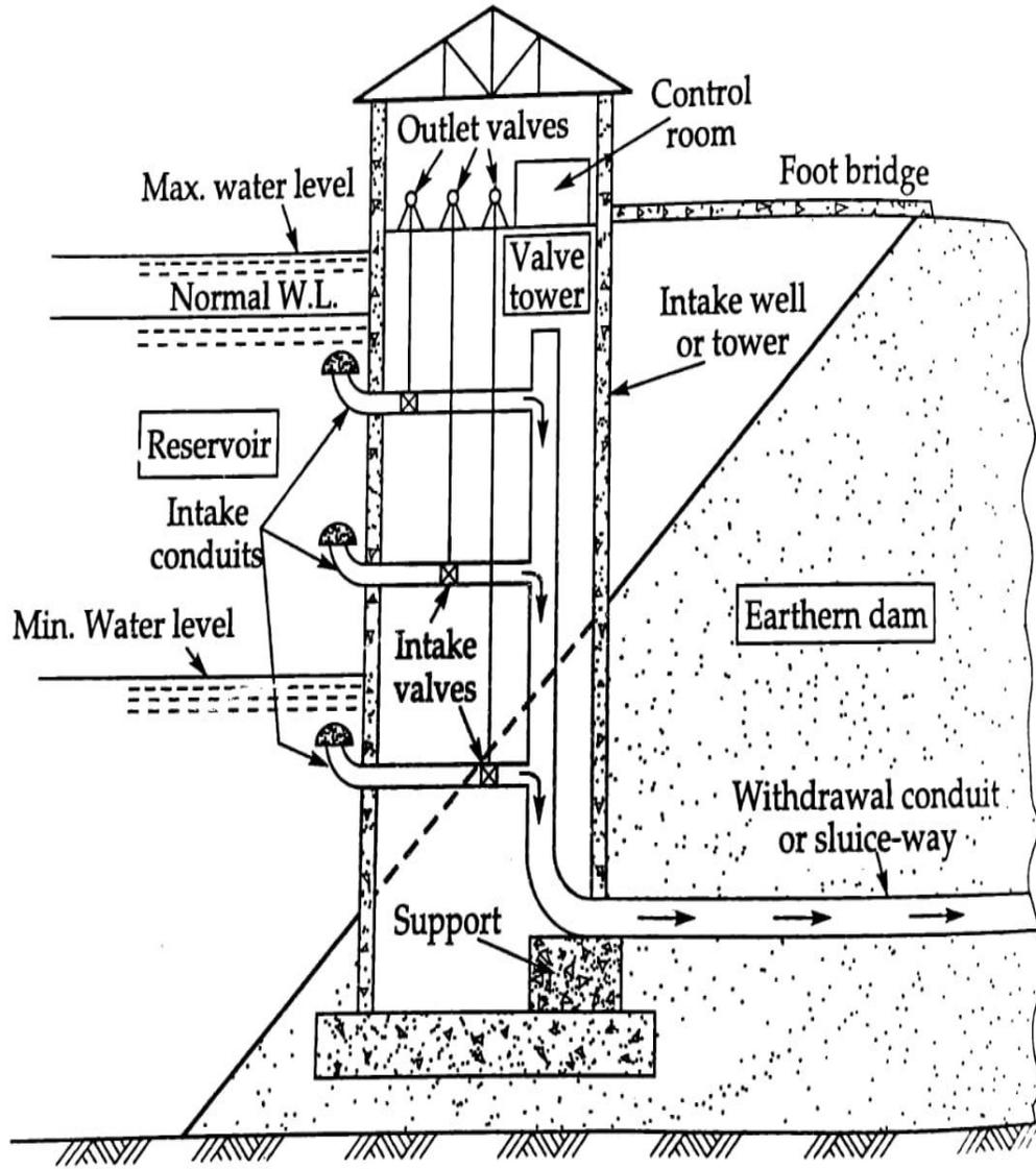
Fig. Valve tower situated at the upstream toe of earthen dam
