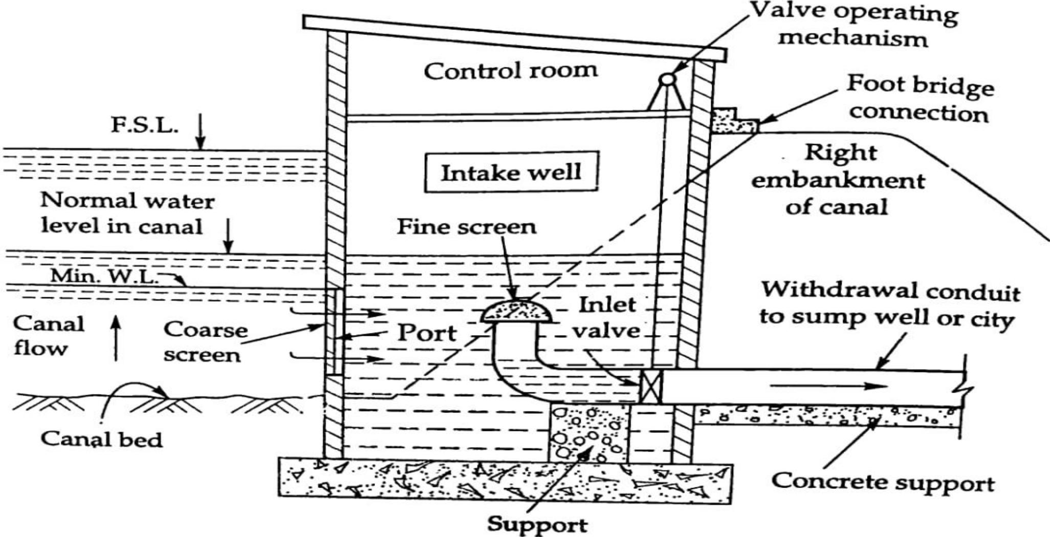
Fig. Canal Intake well
