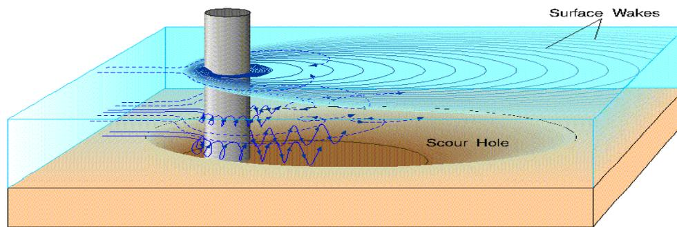
Figure 2.3 Scour hole around the single pile
