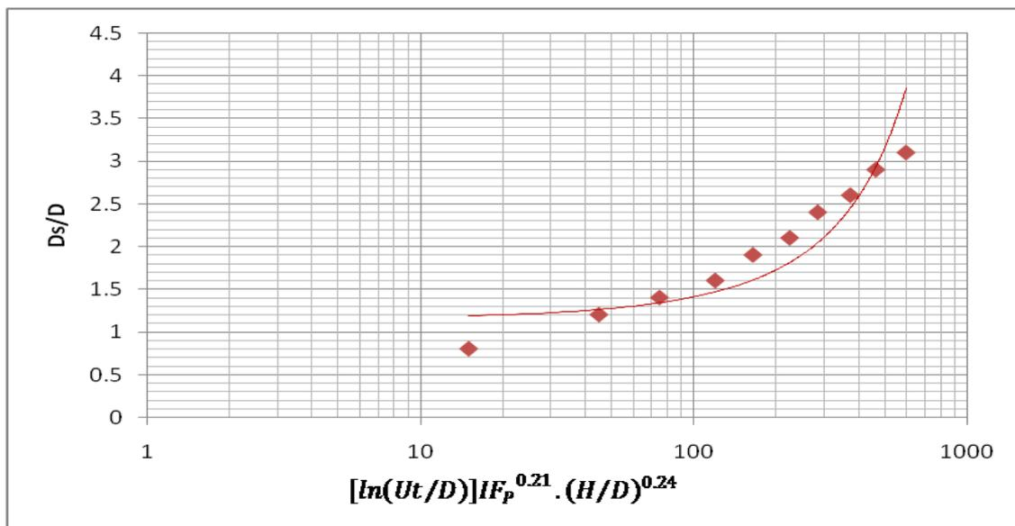
Figure.3.4: Prediction of Scour Depth as a Function of Time
