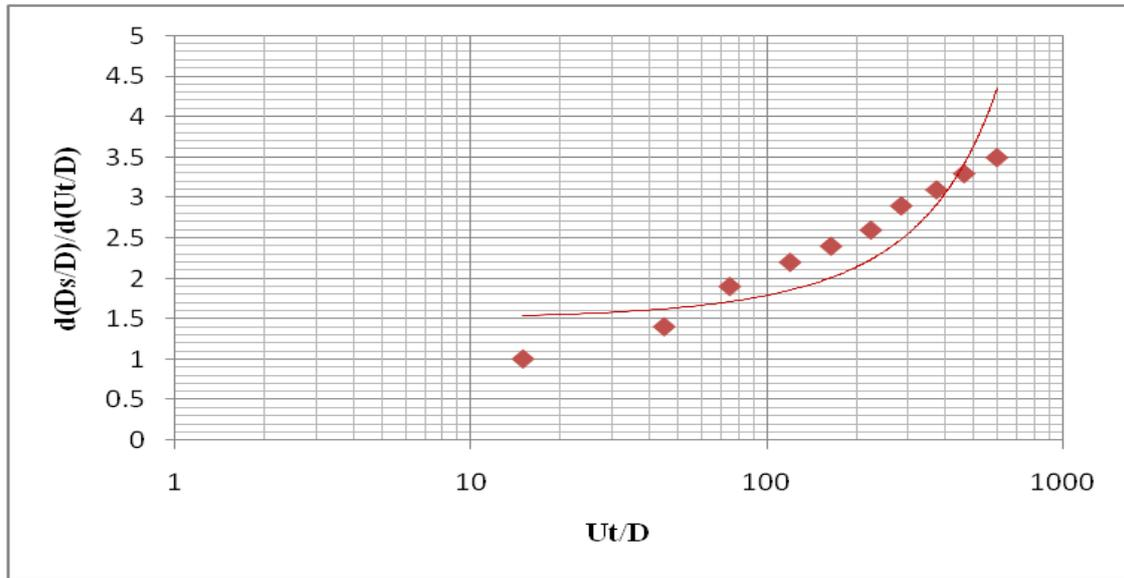
Figure.3.5: Rate of Scour Variation with Time for Fine Sand
