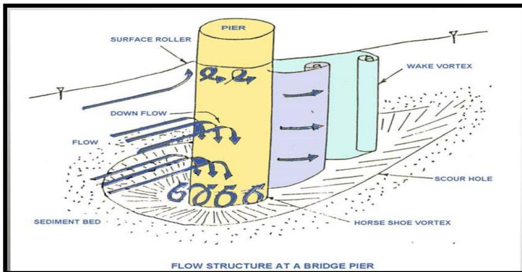
Figure 2.1 Components causing the scouring
