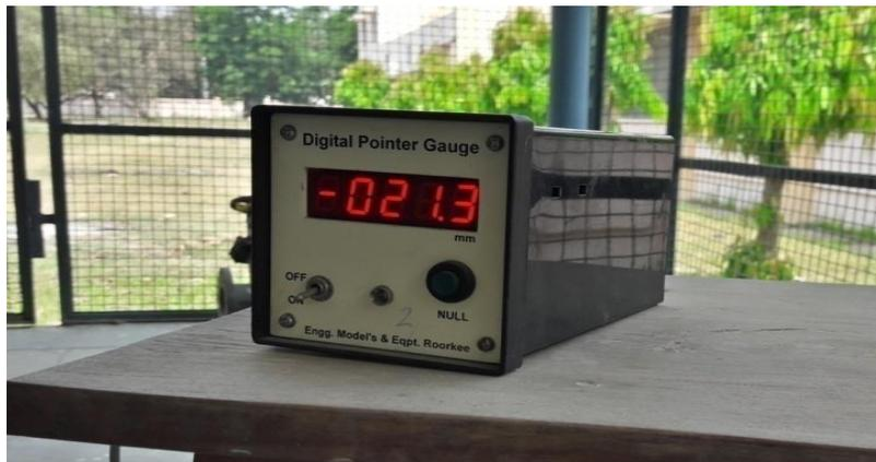
Figure: 3.3 - Digital Pointer Gauge Arrangement
